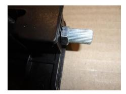
Brake Cable Adjust Studs.
