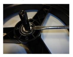
WEAR SAFETY GLASSES WHEN ADDING E-ECLIPS! Use Plyers, or a Flat Head Screwdriver, to add the E-Clip.
