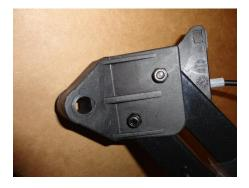
Attach the Brake Housing to the Brake Housing Adaptor using a 10MM Wrench, the remaining Rectangle Head Screw (SV1-208), and two M6 Nylon Nuts.
