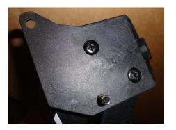
Insert a Rectangle Head Screw (SV1-208) into the inside Rectangle slot of the Brake Housing Adaptor, as shown. Place the Brake Housing Adaptor on the Right Wheel Fitting (005-012R).
