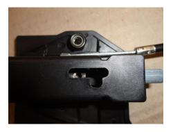
Pull the end of the Brake Cable out of the Brake Cable Sheath as far as possible, then check to ensure the Stud at the end of the Brake Cable will reach beyond the threads in the Brake Pin.
