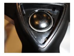
Insert Rear Axle. The O-Rings are tight, and the Axle should be pounded in firmly using a Rubber, or Plastic, Mallet.
