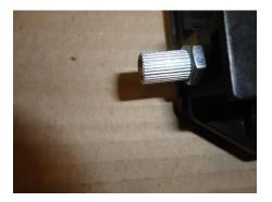
Check to ensure the Upper and Lower Brake Cable Adjustment Studs are screwed all the way in. If not, loosen the Nuts with a 10MM Wrench, twist the Studs in, and retighten the Nuts.
