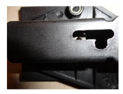
Put the Brake Lever in the 'Brake On' (Down) position. Twist the Brake Pin until you can see the threads in the Brake Pin.
