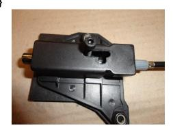
Push the Brake Cable through the Brake Cable Adjustment Stud and into the Brake Pin until the Stud at the end of the Brake Cable is beyond the threads in the Brake Pin.
