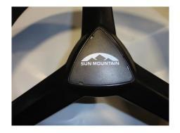
Add Rear Wheel Center Cap. Start the Cap off slightly ajar, then twist it into place.
